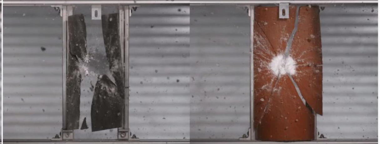
Test video for the highest (class 4) hail rating, filmed at 2,500 frames per second. Each 2" hailstone is travelling 100 mph on impact.
